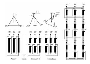
The Figure above shows the schematic of a three- phase transformer with an irregular vector group of Dd11.75 (-7.5°) and Dd0.75 (22.5°).
