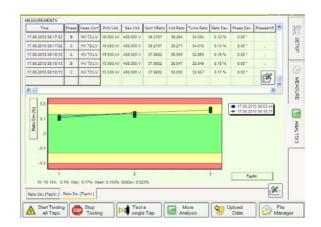
Setups of the TTR 2796 can be stored on, or recalled from the hard-disk or memory-stick. By pre-configuring test setups, the test time during manufacturing or onsite can be greatly reduced. Measurements that are taken onsite and stored inside the TTR 2796 memory can be uploaded at a later moment to a PC via the remote software for more detailed evaluation and analysis of the test results.
