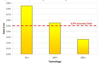
With 250V the measured error is below the 0.5% accuracy limit (red dotted line) specified in the IEC 60076-1 and IEEE C57.12.00-2006-1.
