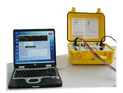
The included TTR APSW 2796 software offers remote setup and control of the TTR 2796 from a computer through a USB connection. Additionally advanced analysis is available like customized graphs, trending and report generation capabilities. Pre-captured measurements as well as live data can be analyzed, stored or recalled.
