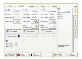
The comprehensive user interface guides the operator through the setup steps by entering nameplate info, transformer vector group, environmental conditions and user comments.
