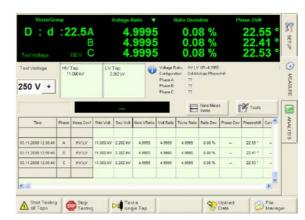
The license enabled APS feature is embedded in the application software. It controls the TTR 2796 through a USB connection from a computer (not included).
