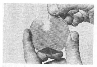
Cut Surface Saver Tape. Lift tape at lens edge adjacent to air bubble to allow escape of air.
