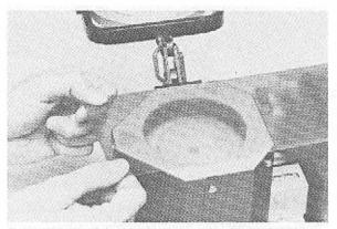
Grasp tape at both edges and pull until the opening over the applicator platen is evenly covered.
