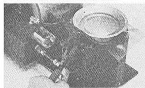
4. Apply tape to lens by closing the applicator cover ring and pushing the applicator clamp lever all the way down to activate the vacuum. (NOTE: See section on special lens procedures for tips on lenticulars, biconcaves, executives, et al.)
