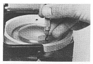
Hold the Surface Saver Cutter blade steady with fingertip to initially penetrate tape.
