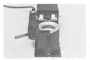
Set the 3M Surface Saver Applicator so that the end with the applicator ring is towards you.
