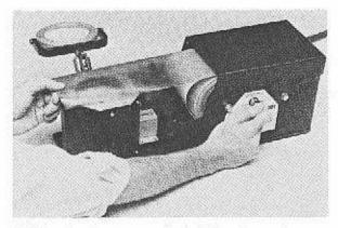
If liner looping occurs, adjust clutch set screw to assure sufficient tension for removal of liner from Surface Saver Tape on the rear core.
