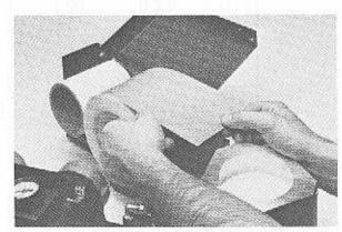
Place the new roll of 3M Surface Saver Tape on the tape reel closest to you with the loose tape end on top pointing toward you.
