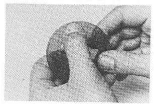
Use thumb pressure in the center of the bubble to force air out from under the tape.
