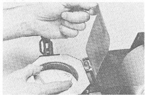
Center lens to be processed on recessed applicator platen.
