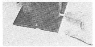
Raise applicator cover ring. Depress reset lever on right side of applicator to lower the applicator platen and prepare unit for use.
