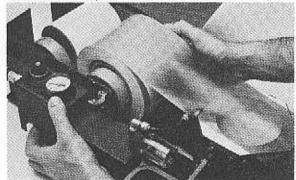
Close applicator sides guiding reels into open ends of tape cores. Close and secure cover with clamp.
