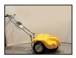
micro GripTester is a cost effective and dynamic alternative to Pendulum spot measurements
